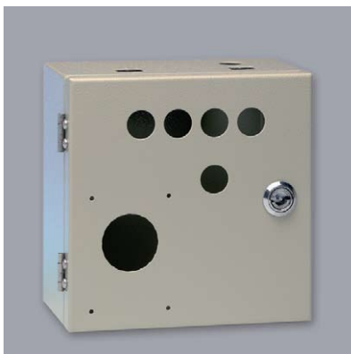
Customer-specific cut-outs are prepared prior to the surface treatment and painting, due to which corrosion resistance remains high, even in the cut-out areas.
