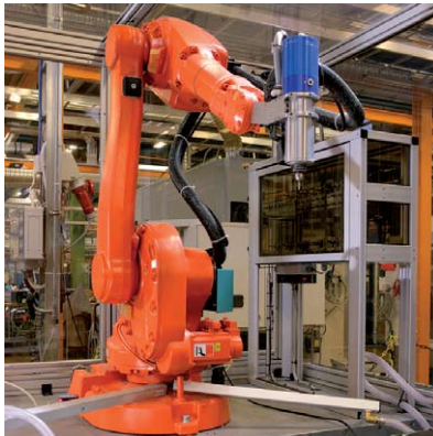
CuboFlex robot cell used for customising thermoplastic enclosures.
